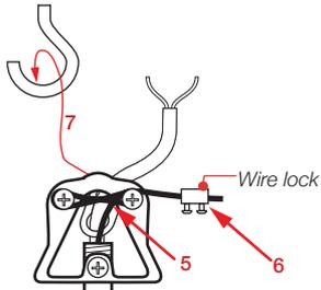
5. Fix the metal wire around the screws on the suspension rod.
