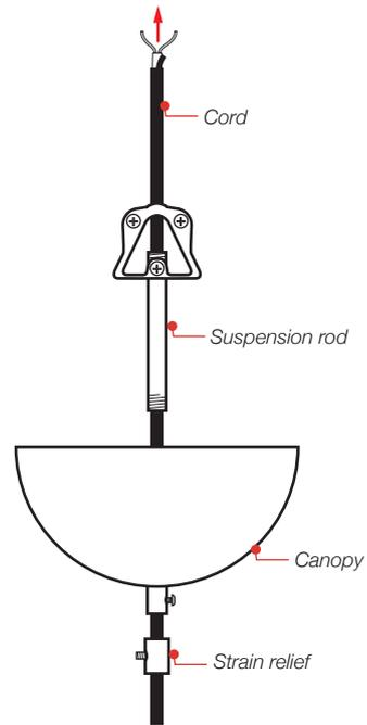
2. Carry the cord through the strain relief, canopy and suspension rod.
