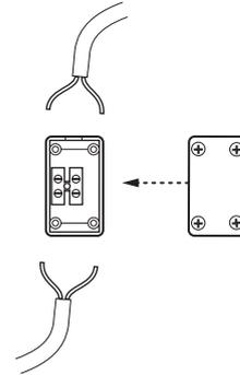
8. Connect the cords to outlet or run it further by using the connector box.
