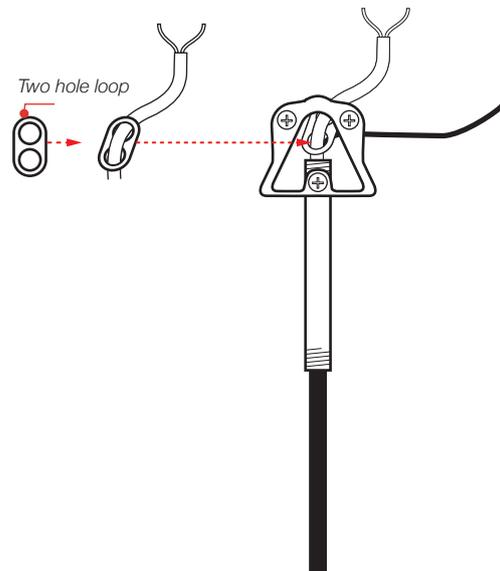
4. Secure the two hole plastic loop to the word - it will make sure it won't slip.
