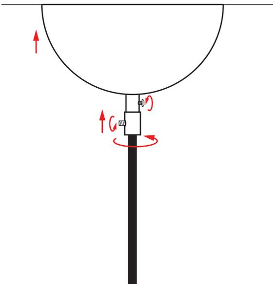
9. Carry the canopy up to the ceiling and tighten the relief screws.
