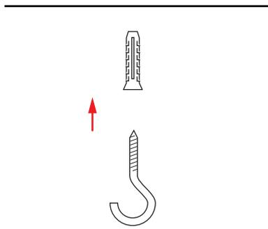
1. Screw the hook firmly into a stable ceiling
