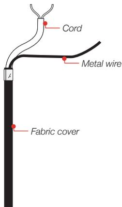
3. Determine at which height the lamp will hang and shorten the cord accordingly. NB! Leave extra cord for power connection and securing of the metal wire.
