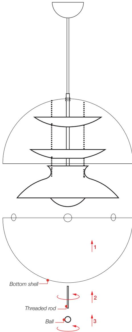
1. Carefully lift the bottom acrylic shell into place.
